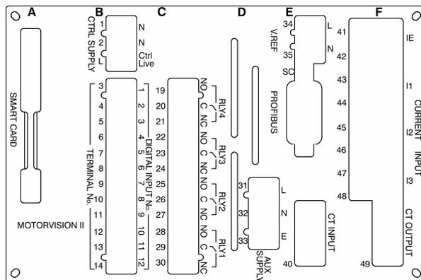
MV2 backplate layout with Profibus Connector
