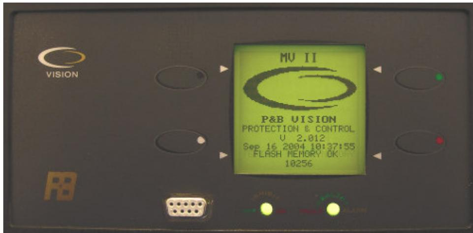
AMV2 or RTDMV2 type display with front mounted RS232 port.
