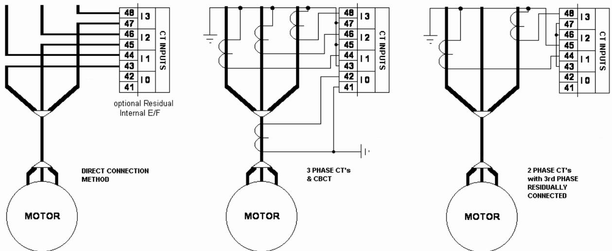
Connection of MV2 to the current measuring circuits can be realised in a number of ways:
