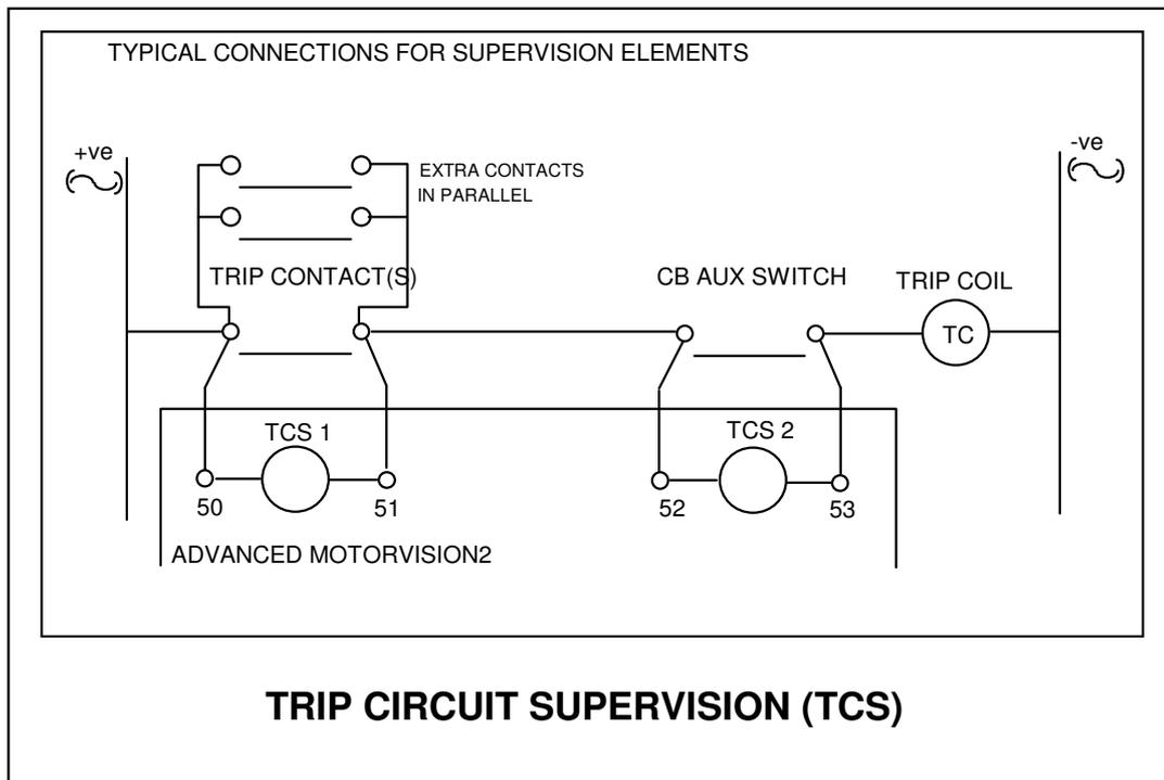
The TCS element consists of two input circuits and two dedicated change-over contact output relays operating in tandem. As the TCS board does not interact with the main relay processor one of the digital outputs provided by the Trip Circuit Supervision should be fed back into the AMV2, as an External Fault input configured to alarm and / or inhibit. The other output can be used to drive an indication lamp for example.
