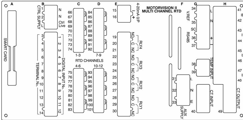
MV2 with multiple RTD Inputs backplate layout with CT card
